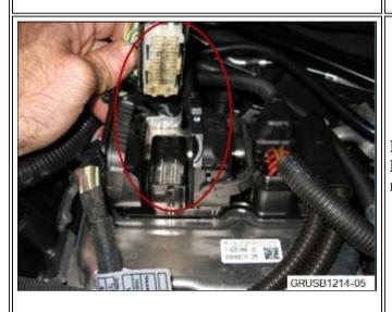
If corrosion or damage is found, the DME and affected engine harness module(s) need to be replaced.
