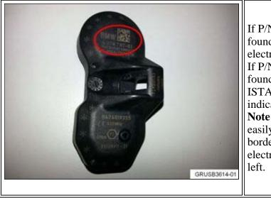
If P/N 4 078 787 or 4 079 152 is found, replace all four wheel electronics with P/N 36 10 6 856 227. If P/N 4 078 787 or 4 079 152 is **NOT** found, proceed as instructed by the ISTA test module and replace the indicated sensor. **Note:** P/N 4 078 787 or 4 079 152 is easily identified by the stars that border the face of the wheel electronics, as seen in the picture to the left.
