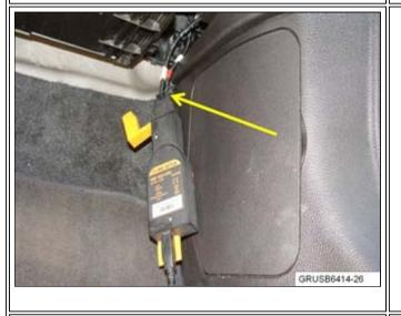
8. Remove the two MOST bus cables from the connector piece. Insert the two cables into ICOM B. Connect the USB cable to ICOM A.
