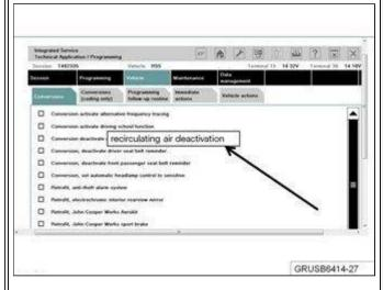
9. To remove this feature, select the conversion "recirculating air deactivation."
