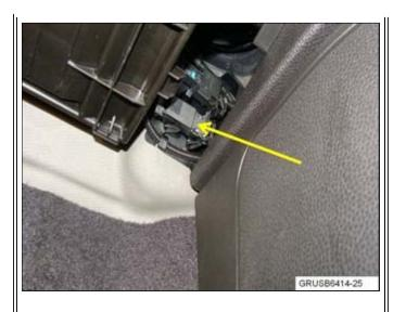
footwell near the bulkhead. Remove the connector piece from the securing bracket.
