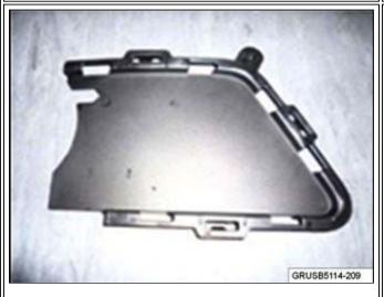
3. Unclip the sealing panel from the air duct by using a suitable pry tool. Discard.
