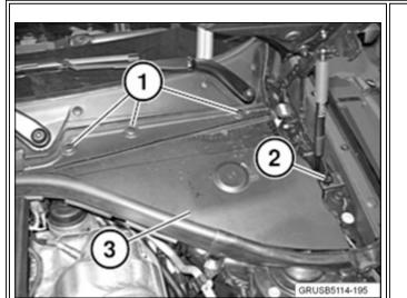
Left side: Turn the locks (1) 90 degrees counterclockwise. Unlock the catch (2) and remove the cover (3).
