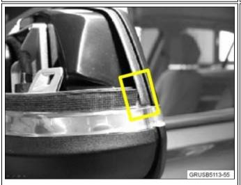
5. Start by applying the tape to the area shown and be careful not to overlap the tape into the area where the mirror cap cover fits.
