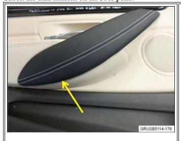
1. Check the lower catch locking by pulling on the trim at the location shown.
