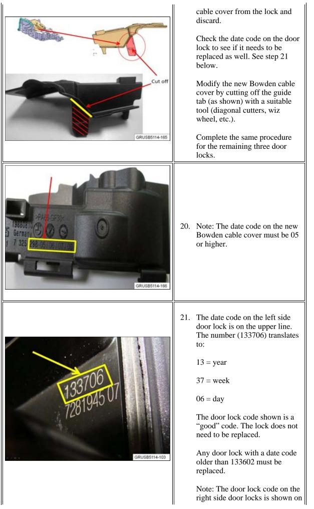
The repairs performed should be four new modified Bowden cable covers on all four doors and replacement of any door lock with a date code older than 133602. Once confirmed, reinstall all removed parts in reverse order of their removal.
