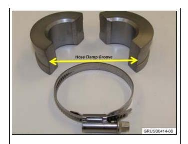
**Note:** The groove in the mass halves is where the hose clamp must be located.
