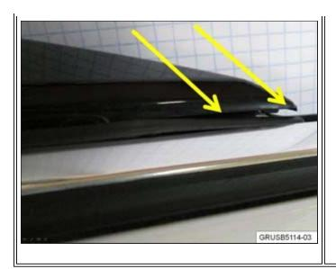
12. If proper fitment of the seal lip to the window frame cannot be achieved (gap showing) after proper seal fitment, replace the mirror assembly. Refer to Repair Instruction 51 16 001, "Removing and installing/replacing mirror on left or right front door" and replace the mirror.
