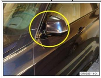
1. Locate the affected mirror or mirrors. Either side mirror or both may be affected. Refer to Repair Instruction 51 16 001, "Removing and installing/replacing mirror on left or right front door" and remove the affected outside door mirror. The ISTA repair instructions are included below.
