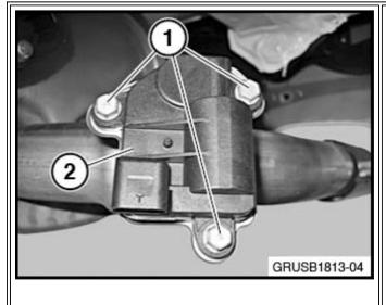
Replace all three screws (1) for the exhaust flap actuator (2). The replacement screws are an improved design.
