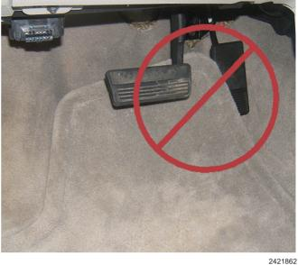
After installing floor mats, make certain they cannot move and do not interfere with the accelerator or brake pedals.
