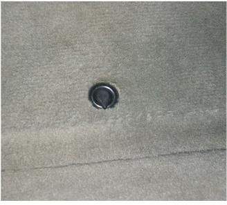
If your vehicle is equipped with a floor mat retaining pin(s) or clip(s), make certain the mat is installed correctly and according to the instructions.
