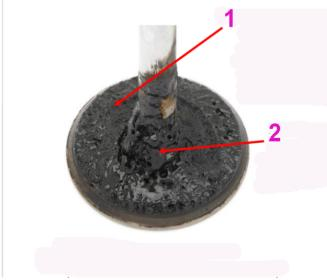
Deposits (1) on the intake valve reduce fuel economy by creating a porous surface that collects wet fuel, thereby affecting the air to fuel mixture in the cylinder and releases fuel late in the combustion cycle leading to increased unburnt hydrocarbon (HC) and carbon monoxide (CO) emissions (2). Likewise fuel injectors may become restricted with carbon deposits over time resulting in an incorrect injector spray pattern and similarly increasing HC and CO emissions.
