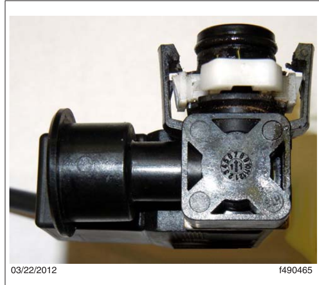
Fig. 2, 10-Watt Solenoid Valve ( 13.5\pm 0.7 \Omega )
