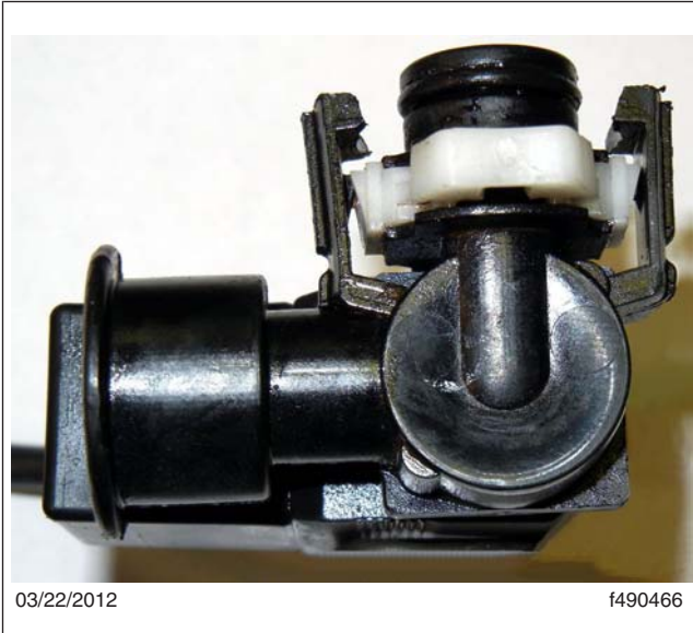
Fig. 1, 7-Watt Solenoid Valve ( 20\pm 1 \Omega )
