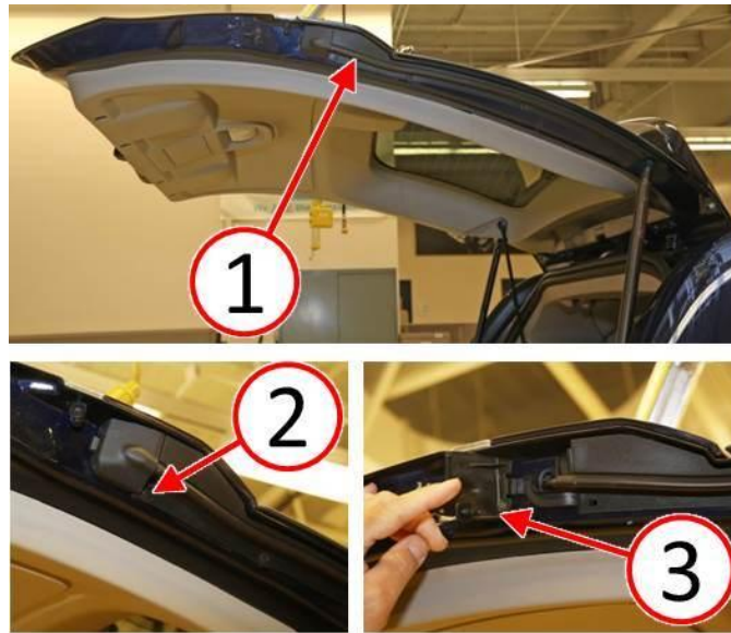
Fig. 1 Liftgate Pinch Sensor Inspection
