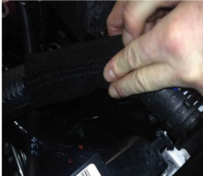
Fig. 15 Kevlar Sleeves Radiator Hose
