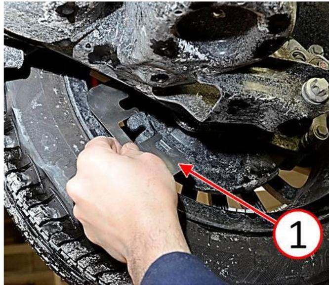
**Fig. 3 Insert Front Shim - Right Side Shown**
