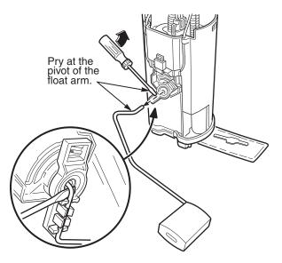
16. Remove the sending unit from the fuel pump assembly:
