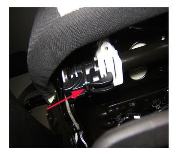
4. Install a nylon wire tie as shown. Trim the excess wire tie material.
