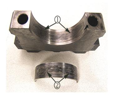
Signs of bearing fretting will also be noticed on the connecting rod and main bearing caps. Refer to the above illustration for fretting of main bearing cap 1 and back side of connection rod bearing 2.
