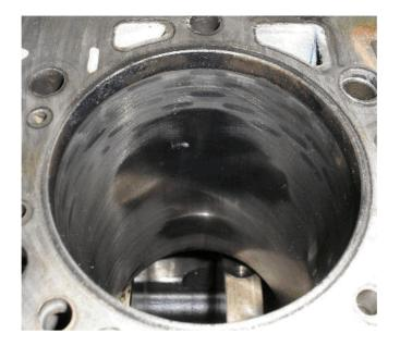
• Crosshatch will be polished off the cylinder wall in the major thrust face of cylinder below ring belt travel.
