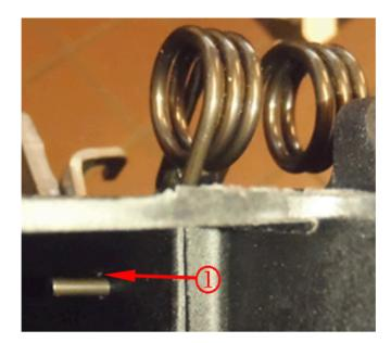
2. Apply GM Super Lube on both sides of the hole on the clutch pedal return spring (1), and both spring coils (2).
