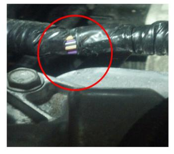
These conditions may be caused by one of the wires (in particular circuits 2500 and 2501) in the engine wiring harness being chafed, cut or damaged due to contact with the right rear corner of the engine or cam/valve cover.
