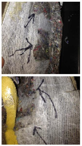
2. Fold back the carpet and remove the insulation from the underside of the carpet to expose the adhesive.
