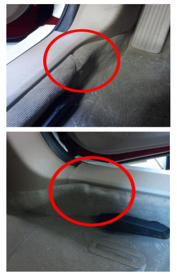
This may be caused by the carpet insulation glued to the back of the carpet not drying smoothly, causing the carpet to appear wrinkled.
