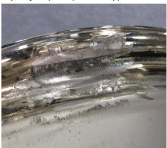
6. Once the corrosion has been eliminated, you should coat the repaired area with a commercially available tire sealant such as Patch Brand Bead Sealant or equivalent. Commercially available bead sealants are black rubber-like coatings that will permanently fill and seal the resurfaced bead seat. At 21°C (70°F) ambient temperature, this sealant will set-up sufficiently for tire mounting in about 10 minutes.
