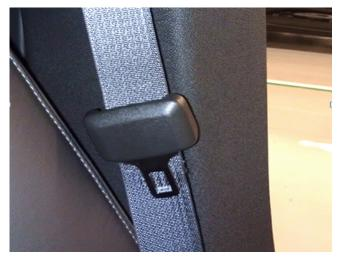
3. When corrected, the latch plate should be in the orientation shown in the graphic above.
