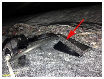
The foam patch on the back of the headliner at the microphone mounting area may have come loose. This foam is a sound barrier for the back side of the microphone. If the patch is detached, it allows unwanted noise to interfere with the microphone operation when making a phone call.
