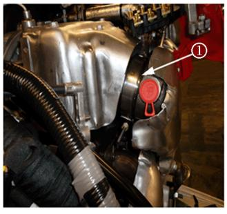
**4.** Remove and discard the exhaust clamp at the turbo to turbo exhaust pipe (1). This can allow the turbo exhaust pipe to be rotated slightly to close the gap as shown in the illustration above.
