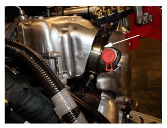
**9.** After alignment of all the joints, install and tighten a new clamp at the turbocharger (if removed earlier).
