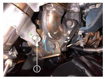
3. If the joint has a gap on either the left or right side, loosen or remove the turbo exhaust pipe mounting bolt (1) as shown in the illustration above.
