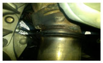
8. Visually verify the joint has good contact completely around the downpipe and the turbocharger exhaust pipe as shown in the illustration above.
