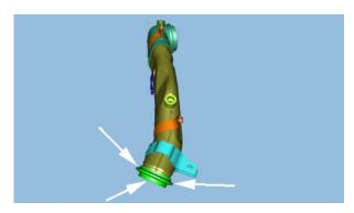
Note: The illustration above is the updated turbocharger exhaust pipe with a pilot flange.
