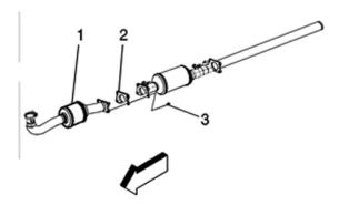
5. Loose or disconnect the four flange mid-joint bolts located after the catalytic converter.
