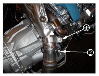
2. Remove and discard the exhaust clamp between the downpipe and the turbocharger exhaust pipe (2) as shown in the illustration above.
