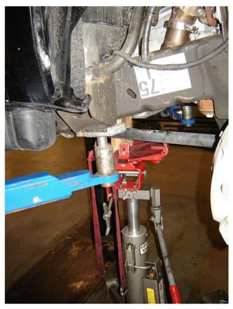
7. Using a transmission jack, align the exhaust pipe, downpipe and the turbocharger exhaust pipe flanges until all mounting joints and the flanges are flush and parallel with no or minimal load or force applied. This could include adjusting the mounts as necessary, allowing the flanges to sit flush with the exhaust in a neutral state, using care not to compromise clearances around the exhaust.
