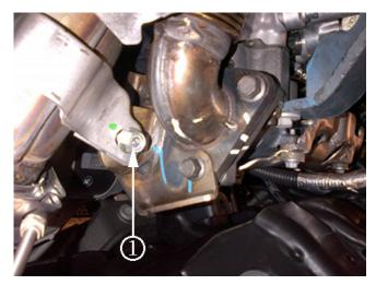
12. Install the mounting bolt (1). If the mounting bracket was removed, align and install the bracket. If the bolt will not line up, bend or shim the bracket until alignment is possible.
