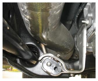
6. Verify that the exhaust pipe hanger at the transmission is mounted in the outer insulator hole as shown in the illustration above.
