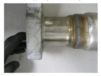
This can be inspected easily by placing a gauge block flush against the flange and inspect for excessive gaps or damage to the flange.
