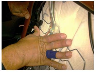
**15.** Reattach the J-clips and the bottom velcro of the inboard side seat cover to the seat frame.
