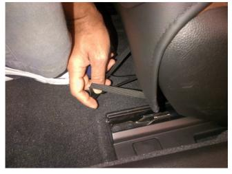
**3.1.** Remove two clips retaining the elastic straps on the toe-kick flap from the underside of the seat cushion.
