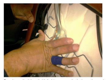
**4.** Pressing on the inboard side bolster, remove the bottom velcro and detach the J-clips retaining the seat cover to the seat frame. Detach the clips from top to bottom to gain access to the bolster solenoid fastener.
