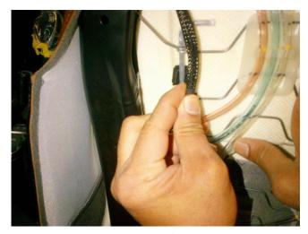
7. Detach the wire harness routing clip from the lumbar suspension wire to make room for solenoid removal.
