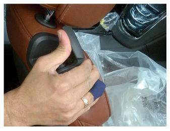
1. Recline the seat back forward by lifting the seat back lever.
