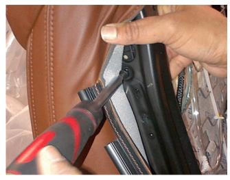
**6.** From the left outside of the seat back, remove the T20 torx screw retaining the bolster solenoid to the seat frame bracket.
