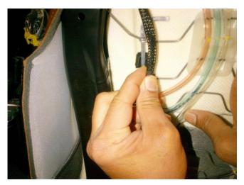
**14.** Reattach the wire harness clip to the lumbar suspension wire.
