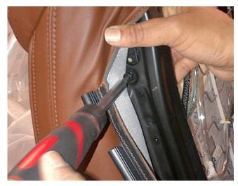
13. Reposition the solenoid to the seat bracket and install the torx screw. Tighten to a maximum of 2.5 Y (22 lb in).
