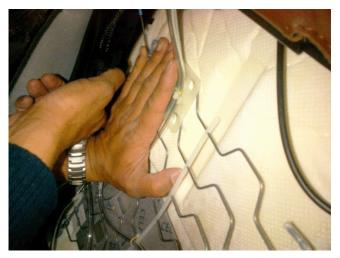
9. Slide the solenoid upward slightly to disengage the hook feature and position the solenoid/hoses outside the seat frame.
