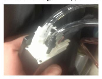
Note: Use "Push / Pull / Push" method to remove and reinstall the hose.
