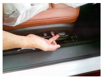
**2.** Adjust the seat to the most upward position by pushing the up/down button switch.
