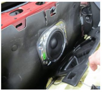
7. Remove the four nuts securing the sub woofer.
