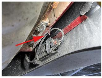
Position the harness outboard of the rear compartment floor lower extension as shown. It may be necessary to loop the wiring over itself and secure with a wire tie to take up any excess slack in the wiring.
