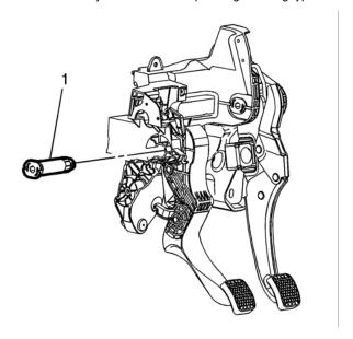
This may be caused from lack of or no lubrication on the clutch pedal pin (1) shown in the illustration above.
