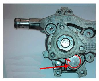
3. Apply a small bead of RTV Engine Sealant, P/N 88864346 (in Canada, P/N 88861418) to the seam around the perimeter of the reservoir cup plug. Be careful to avoid plugging the small hole at the top of the reservoir with the sealant. This evaporation hole must be left open.
