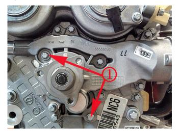
Tighten these two fasteners an additional 30 degrees (1).
