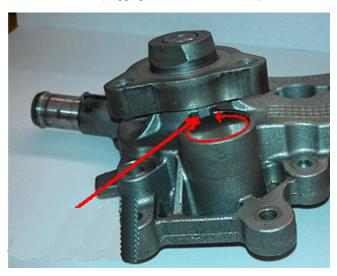
4. Use a clean scraper to work the sealer into the cup plug gap and to scrape off any excess leaving a thin layer to seal the cup plug.
