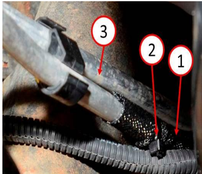
Fig. 5 Transmission Oil Cooler Tube Sleeve
