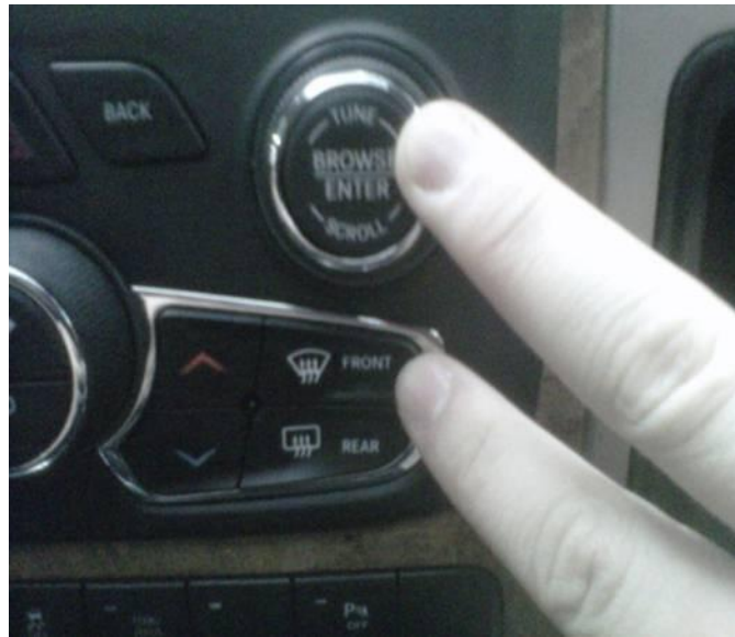
Fig. 2 Take Vehicle Out of Ship Mode
