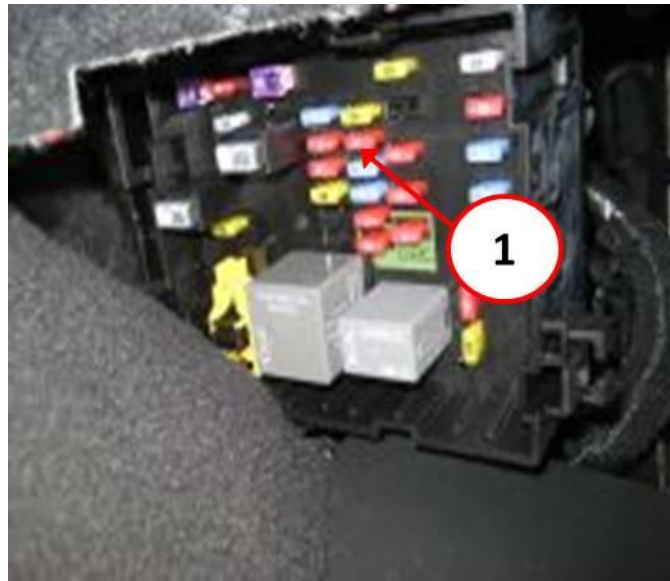
Fig. 4 JC Passenger Side Fuse Block
