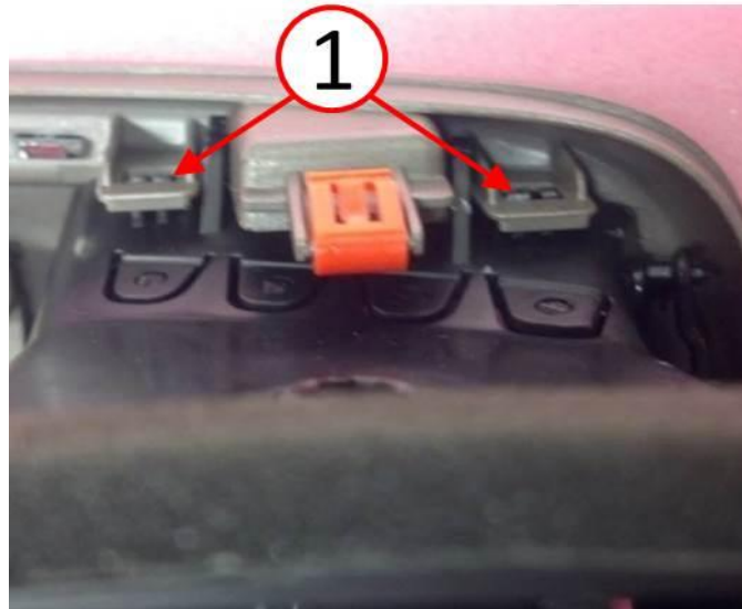
Fig. 3 HVAC Outlet Upper Attachment
