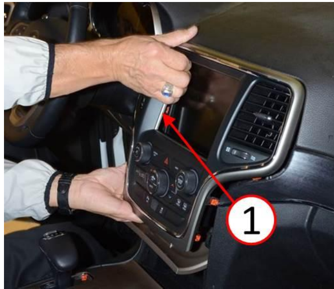
Fig. 11 ICS Bezel Removal Upper
