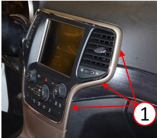
Fig. 15 ICS Bezel Installation Inspection
