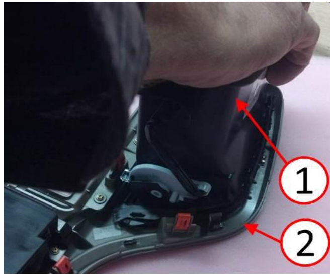
Fig. 4 HVAC Outlet Lower Attachment
