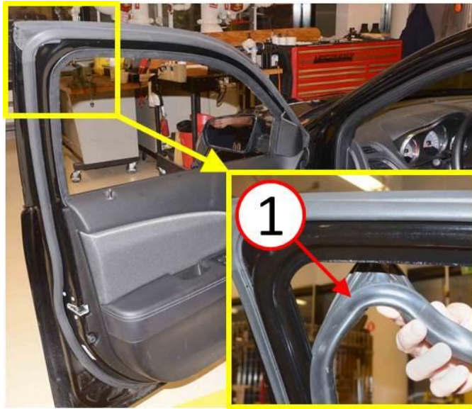
Fig. 1 Remove Window Run Channel Seal
