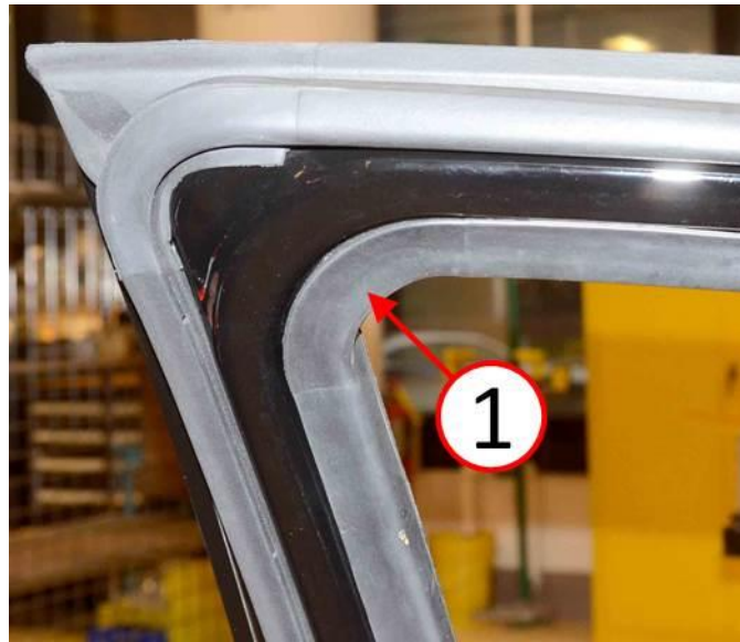
Fig. 5 Install Run Channel Seal
