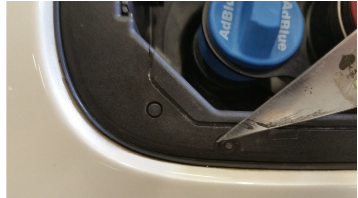
Cut rubber spacer flush with surface
