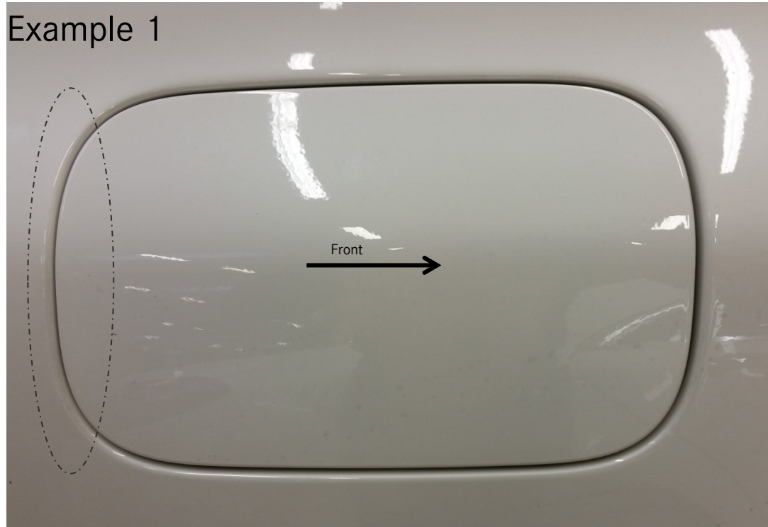
Incorrect spacing at rear
