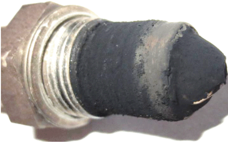
Soot Covered HO2S
