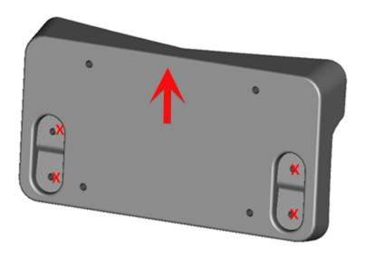
2. Install bolts through the license plate bracket and fascia holes.
