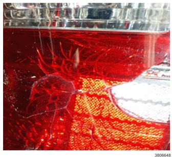
This lamp shows impact damage and internal cracking of the lens.
