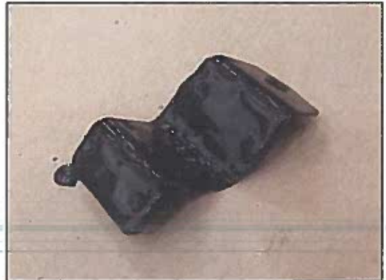
Figure 14. Adhesive Applied to Top of Horn Mounting Bracket No. 3
