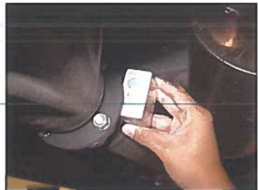
Figure 13. INCORRECT Placement of Protractor
