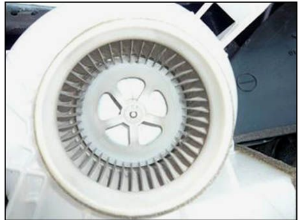
Figure 2. HV Battery Cooling Fan AFTER Cleaning
