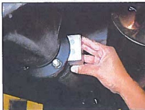
Figure 12. CORRECT Placement of Protractor
