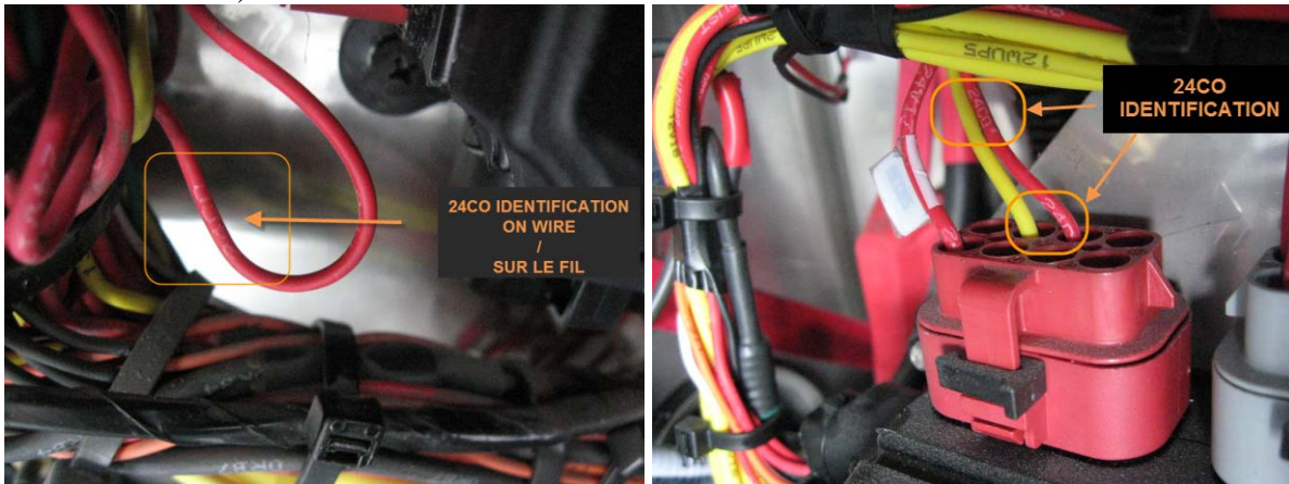
Fig.6 24CO Wire identification on H series (Left) and X series (Right) vehicle.
