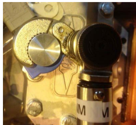
Figure 1 Torque Wrench Position For Setting Torque
