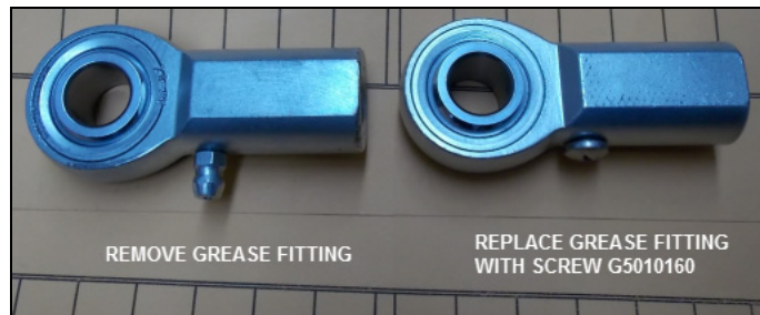
FIGURE 6: FILL ROD END WITH FRESH GREASE THEN REPLACE GREASE FITTING WITH SCREW G5010160
