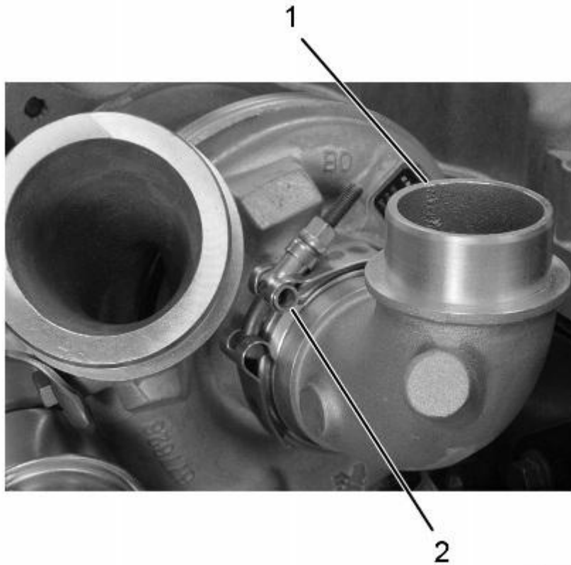
Figure 6. Turbocharger Inlet Elbow.
