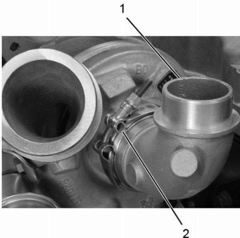
Figure 18. Turbocharger Inlet Elbow.
