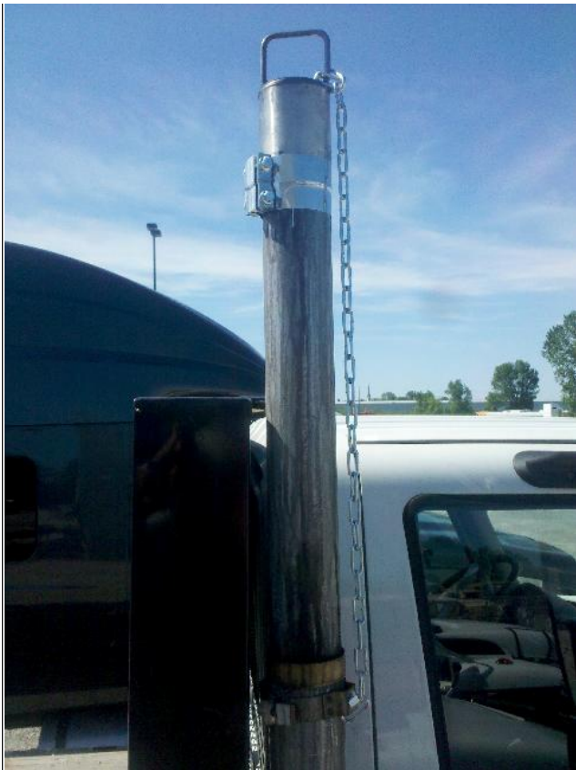
Photo 2 - Vertical Exhaust Restrictor- Chain must be taut and securely attached at the bottom
